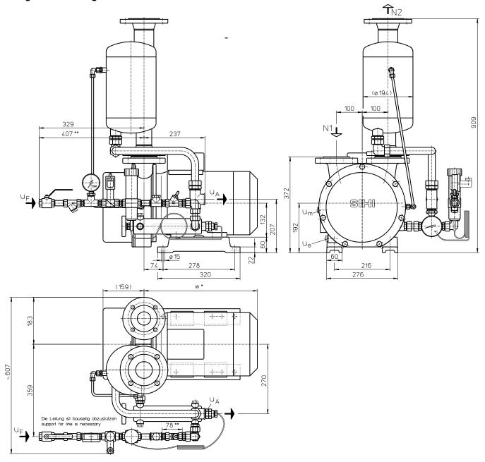
N 1 = gas inlet DN 50 N 2 = gas outlet DN 65 $u_A = liquid drain G 1$
