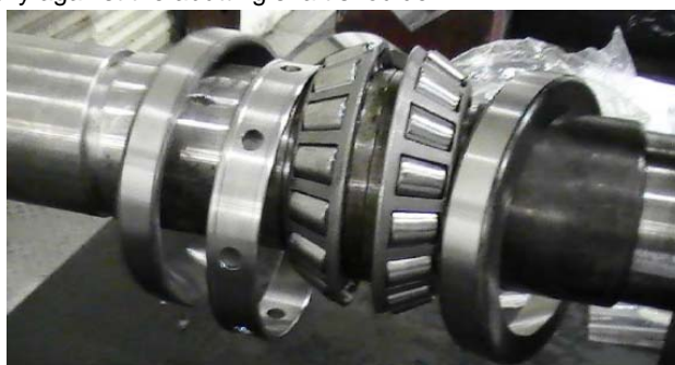
Spacer Ring between two bearing cups
