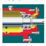
**Hook Sleeve** and replaceable metallic impeller spacer have gasket seals to isolate shaft and impeller threads from slurry. This design extends component life and eases impeller removal.
