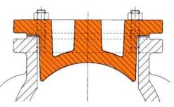
The pump casing is designed with an access hole that permits internal inspection of the impeller.
