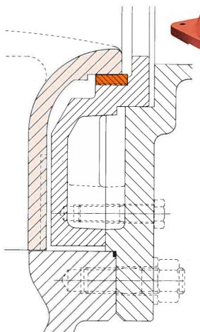
The clearence between impeller and wear plate is kept to a minimum in order to avoid accumulation of sollids.
