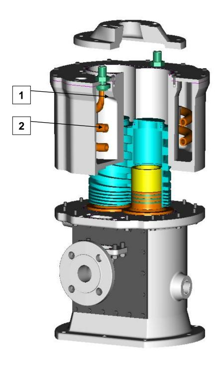
Indirect cooling of the working chamber:
