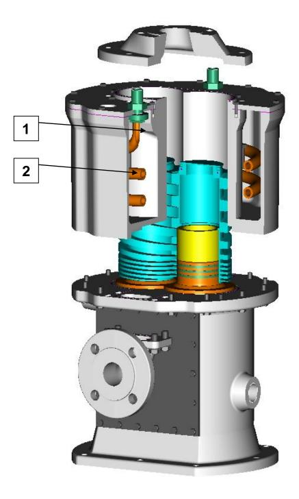
Indirect cooling of the working chamber:
