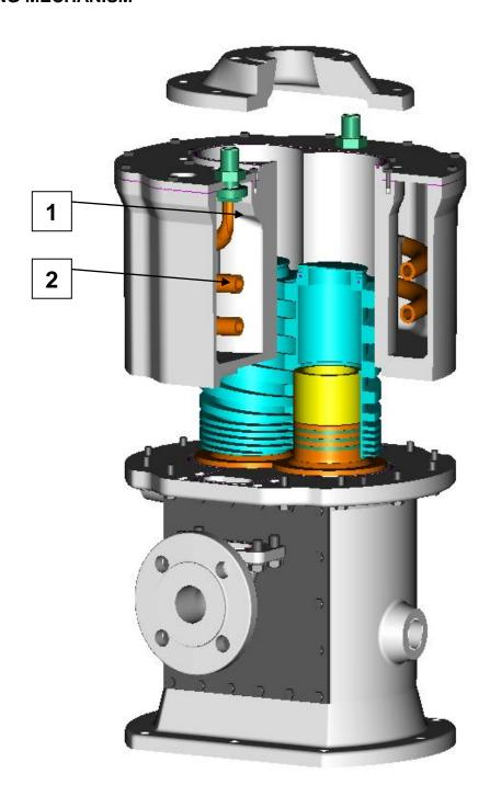
Indirect cooling of the working chamber:
