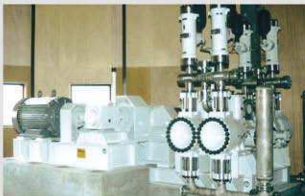
DG 180/200 - 2 K 140 - 4 SM 350 HD Q = 28 m 3 /h p = 150 bar P = 200 kW Medium: H 2 O + organic + inorganic matter
