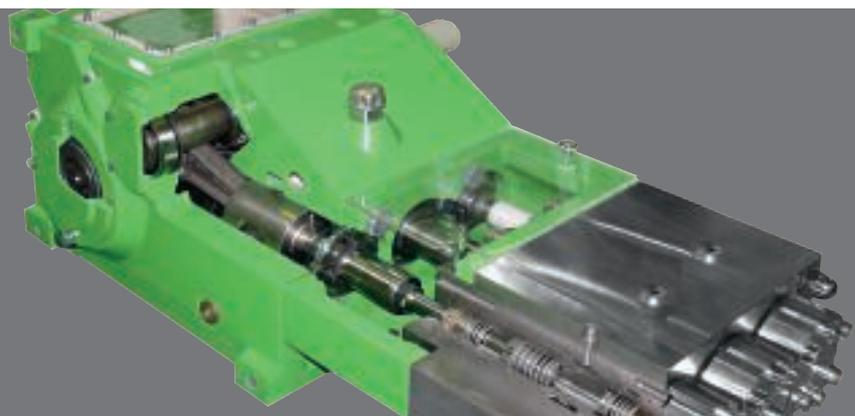
With integrated gear reduction and compact dimensions, KAMAT high-pressure pumps are the ideal tool for numerous applications. Simple operation and maintenance are defining features of KAMAT plunger pumps, as are high modularity and flexibility in regard to delivery rates, pressure settings and fluids. For operating pressures from 0 to 3,500 bar, the input power ranges from 45 to 1,200 kW.
